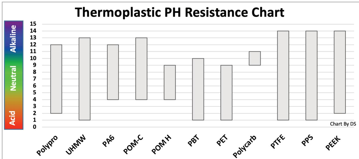
While some of these materials have similar resistance to chemicals, additional factors must be considered when choosing compatible materials. The concentration of chemistry, frequency of exposure, surface finish, pressure, and temperature factor into the part's overall performance and life.
